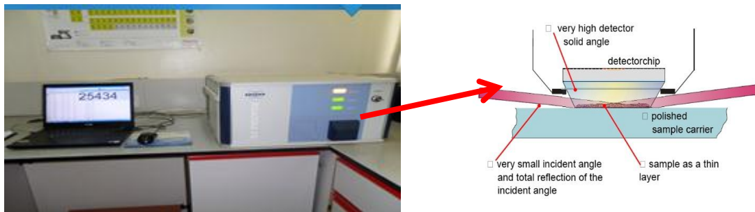
Figure 3.8: TXRF (Bruker S2 picofox) at Institute of Nuclear Science and Technology and schematic presentation of the applied irradiation principles.
