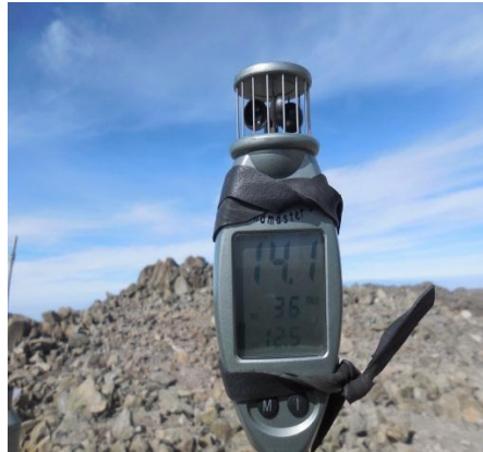
Figure 3.6: An anemometer indicating current, maximum and average wind speed in \text{m s}^{-1} .
