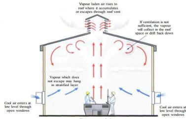
Plate. 2.05: An example of stack ventilation to remove vapours through roof ventilators. (Source: <u>www.ucu.org.uk</u>, 2000)
