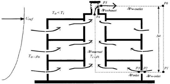
Wind+Buoyancy-Driven Stack Ventilation
