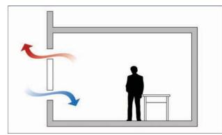
Plate. 2.03: Single sided ventilation. (Source: <u>www.bsria.co.uk</u>, 2009) Where ventilation openings are provided at different heights within the façade, the ventilation rate can be improved by the buoyancy effect. The contribution from thermal buoyancy depends on the temperature variance between the interior and the
