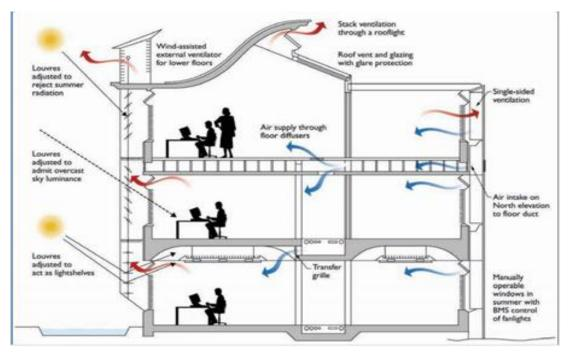
Plate. 2.02: A schematic showing the various natural ventilation strategies. (Source: <u>www.bsria.co.uk</u>, 2009)
