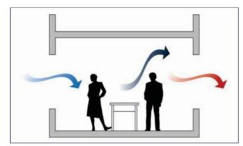
Cross ventilation is also mentioned when considering a single space where air goes into one side of the space and leaves from the opposite side. In this situation the ventilation principle on the system level can be either cross- or stack ventilation. As the air circulates across a fully occupied space, it
