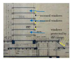
Plate. 4.06: Section through the ICEA building showing air flow. (Source: Architect,2016)
