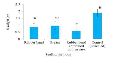
Figure 4.2. Weight loss (%) incurred in metal silos sealed with different sealing methods after 35 days
