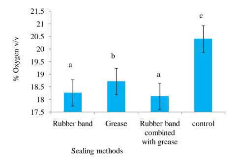
Figure 4.3. Mean oxygen levels in metal silos sealed with different sealing methods after 35 days
