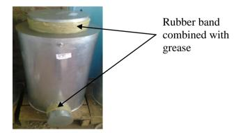
Plate 4.7 One hundred kilogram metal silo with the in-let and out-let sealed with rubber band combined with grease (T3)
