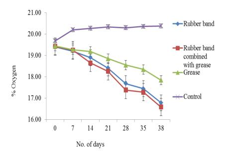
Figure 4.4. Weekly oxygen trend in metal silos sealed with different sealing methods after 35 days
