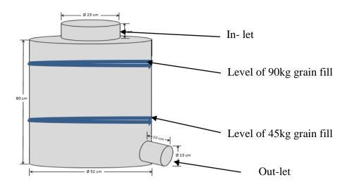
Figure 4.1. Metal silo with a holding capacity of 100 kg of grain
