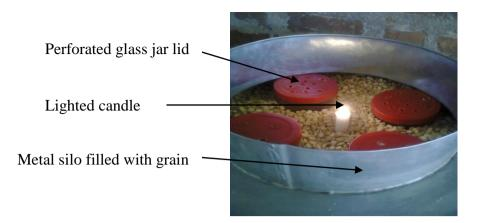
Plate 4.3 Maize in metal silo with a lighted candle next to aerated 1.5 litre glass jar
