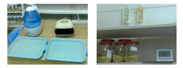
Plate 3.2 Humidifiers, heaters and thermometers in the incubation room
