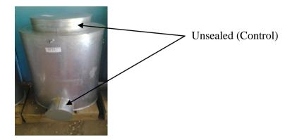
Plate 4.8 One hundred kilogram metal silo with unsealed in-let and out-let (control) (T4)
