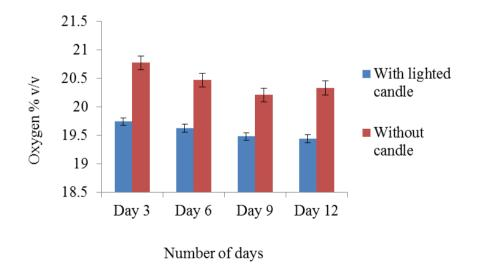
Figure 5.2. Oxygen level in metal silos with and without lighted candle on the third, sixth, ninth and twelfth day
