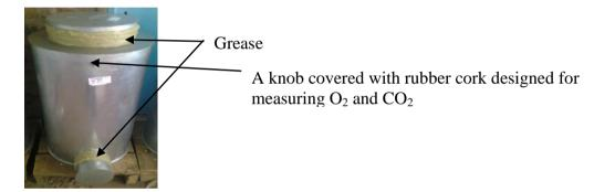
Plate 4.6 One hundred kilogram metal silo with the in-let and out-let sealed with grease (T2)
