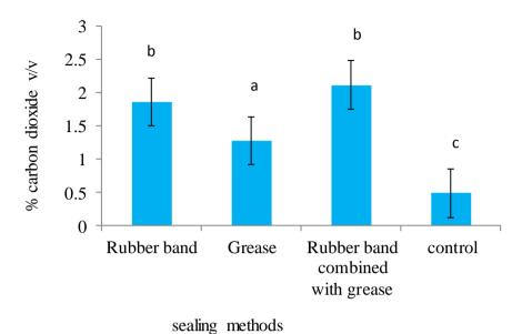
Figure 4.5. Mean carbon dioxide level in metal silo sealed with different sealing methods after 35 days
