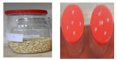
Plate 4.1 One and a half (1.5) litre glass jar with 400gram of grain (right) covered with a perforated lid(left).
