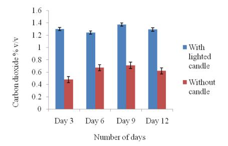
**Figure 5. 1.** Carbon dioxide level in metal silos with and without lighted candle on the third, sixth, ninth and twelfth day.
