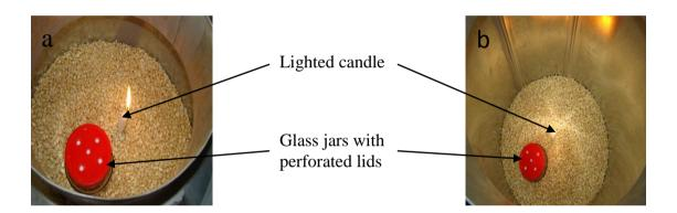
Plate 5.1 Metal silo with a lighted candle next to an aerated glass jar with (a) 90 kg of grain (T1) and (b) 45 kg of grain
