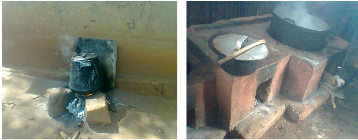
Plate 2: Inefficient cook stove versus efficient energy saving stove (Rocket stove) Source: (Researcher 2014)
