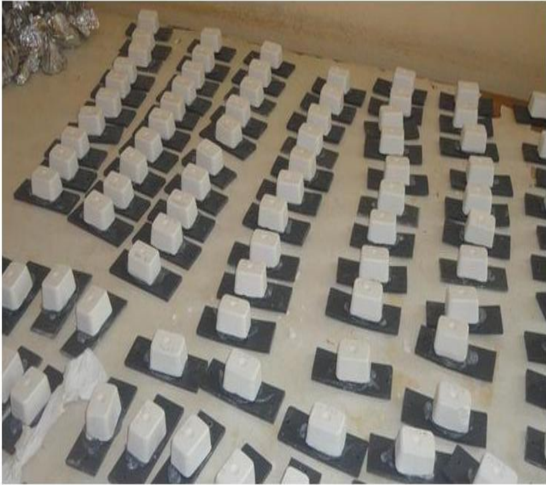
Figure 4: Oven dried clod cards glued on plastic plates with silicon cement before exposure in the field (Photo by David Maina)
