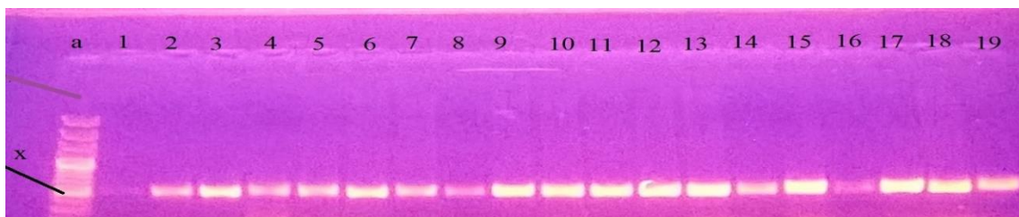
Figure 5. Image of 500bp PCR products run on 1% agarose gel. Lane a is the molecular ladder lane, x is the 500bp marker of the 1kbplus molecular ladder. 1-19 represents PCR samples from Athi River.
