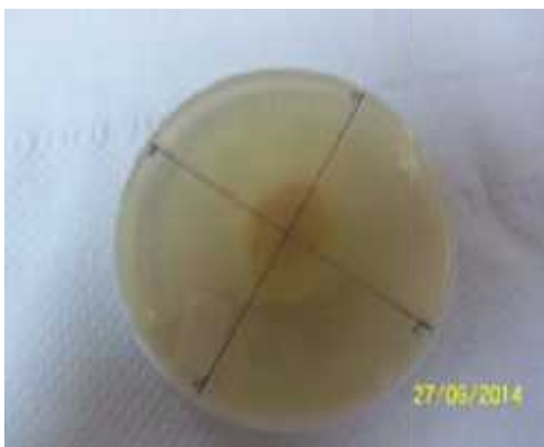
Plate 6: Two cardinal diameters previously drawn on the bottom of each petri dish through two orthogonal axes
