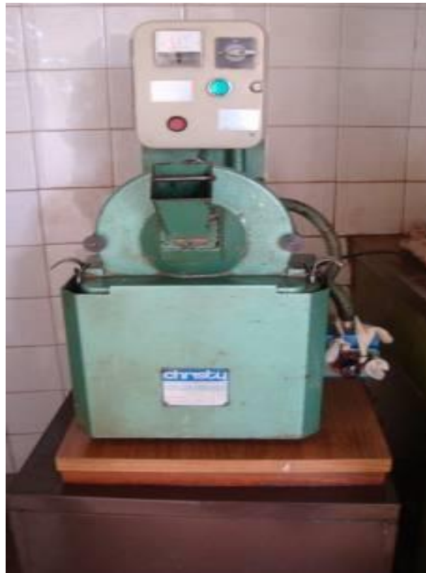
Grinding machine used to grind dried plant materials
