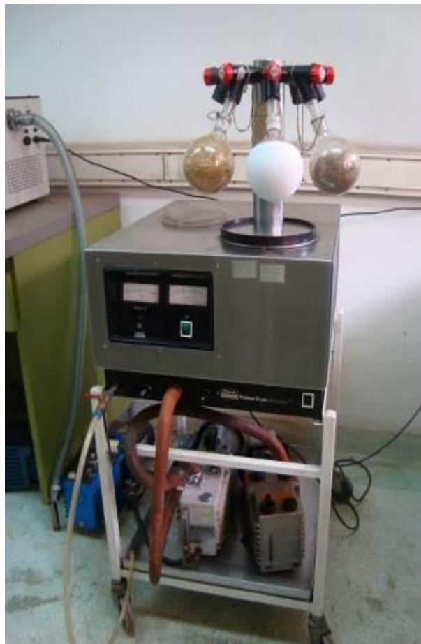
Freeze drying of aqueous crude extract using Edwards Freeze dryer, Modulyo
