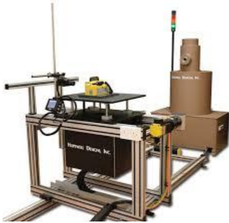
Figure 3.3.: Model GC60 Gamma Beam Irradiator at KBS
