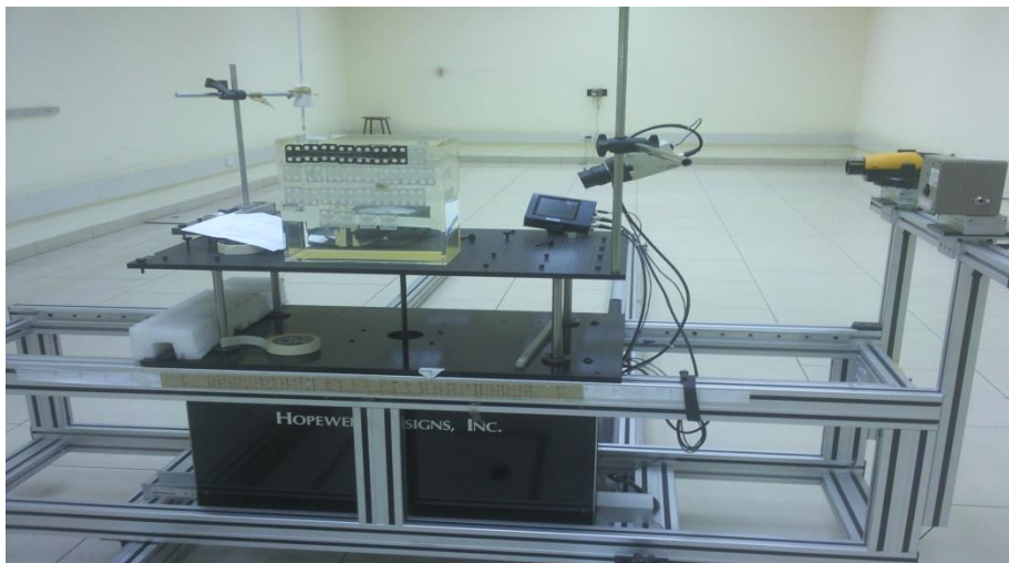
Figure 3.4: Positioning of TLD cards on the polystyrene piece during irradiation
