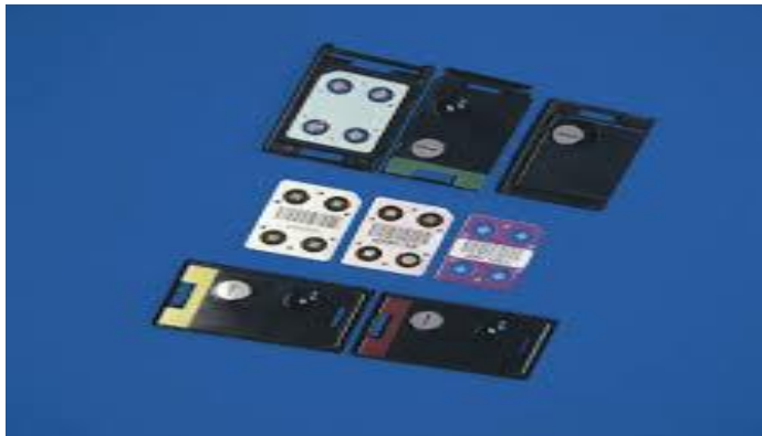
Figure 3.2: Sample TLD 200 cards and holders
