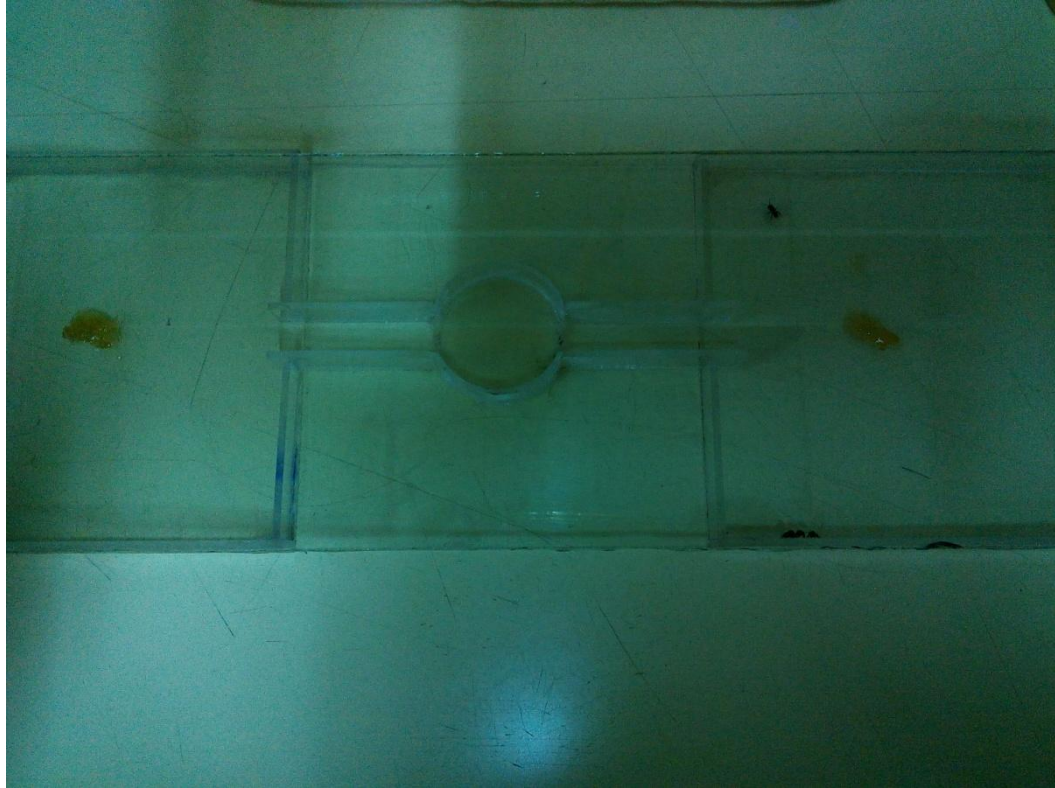
Figure 7.3: Dual choice test bioassay Perspex platform provisioned with both baited (treatment) and un-baited food resource (positive control).
