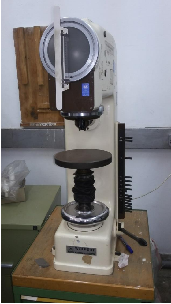
Figure 18: Vickers Hardness Tester (Amsler Otto Wolpert-Werke GmbH D-6700 Ludwigshafen/Rhein) used in this study.
