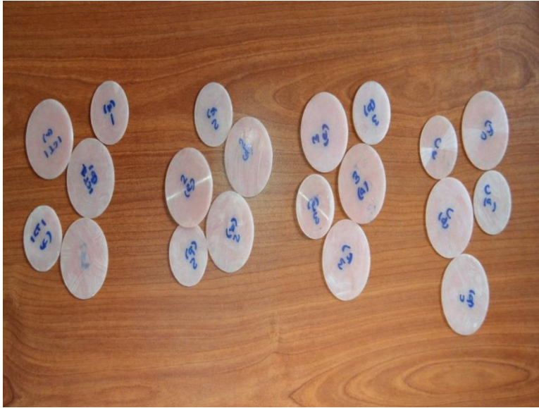
Figure 11: Specimen discs for water sorption and solubility evaluation.
