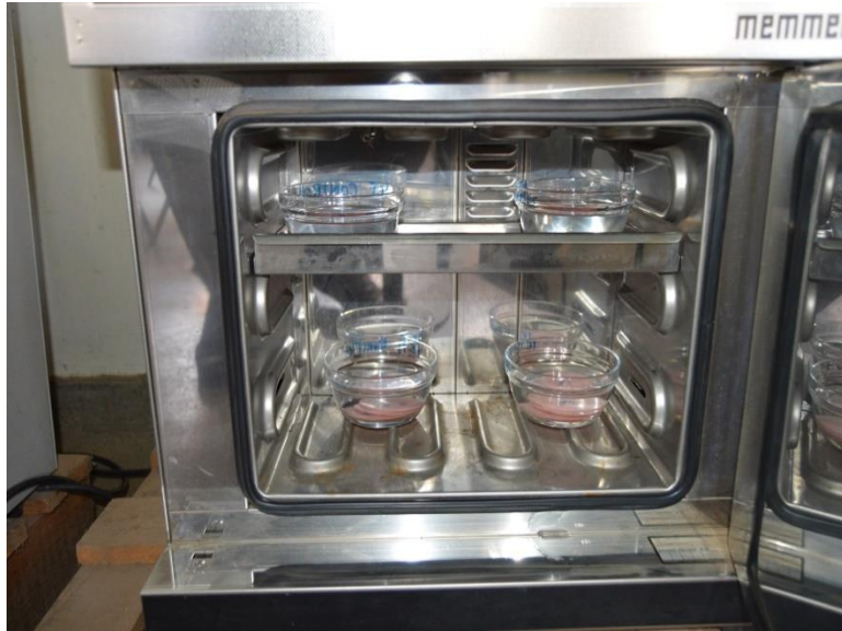
Figure 16: Specimens immersed in distilled water in the oven.
