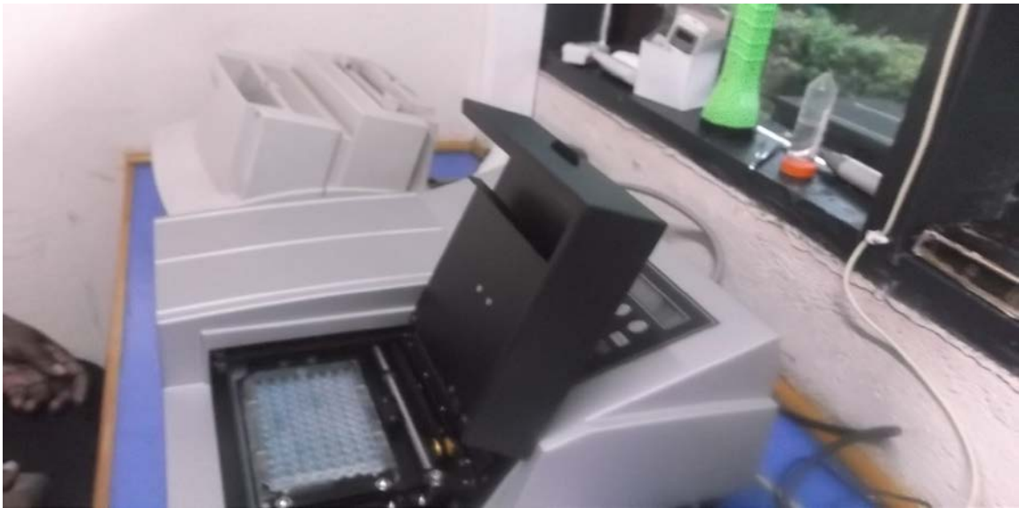
Figure 17: Elisa reader with microtiter plate
