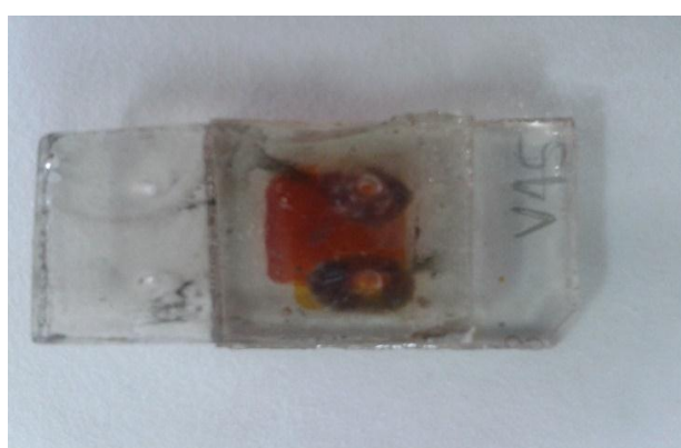
Figure 4.5: Photograph of the assembled dye-sensitized solar cell based on \text{TiO}_2/\text{Nb}_2\text{O}_5 composite electrode film showing predrilled holes through which electrolyte was injected to cell.
