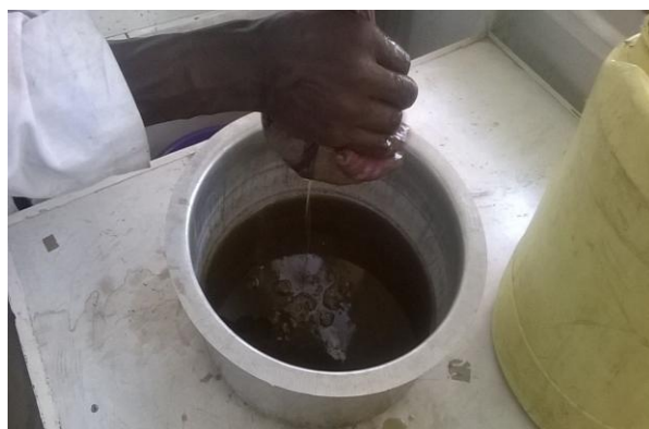
Figure 3.1: Filtration using a modified muslin cloth
