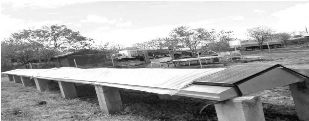
Figure 5.1: Pictorial view of the solar tunnel dryer from the collector end.
