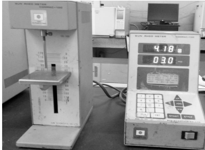
Figure 6.2: Front view of a rheometer equipped with a cylindrical probe after instrumental setting.
