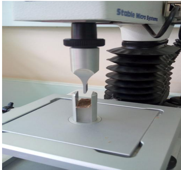
Figure 6.1: Front view of TA.XT. plus Texture Analyser showing the position of the sample between the upper and lower jaws of the volodkevich bite jaws cell.
