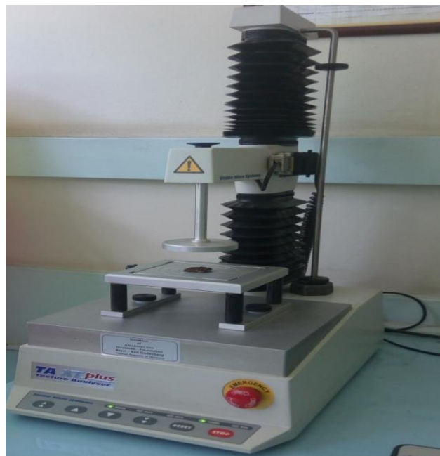
Figure 6.3: Front view of the Texture Analyzer showing the mechanism of compression.
