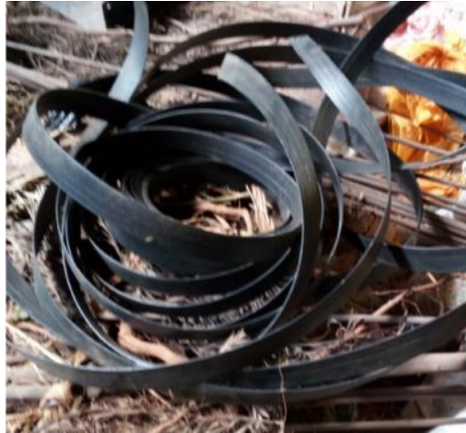
Plate 3-5: Geosynthetic material used
