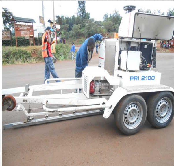
h- Sensors of FWD touching the ground & ready for testing
