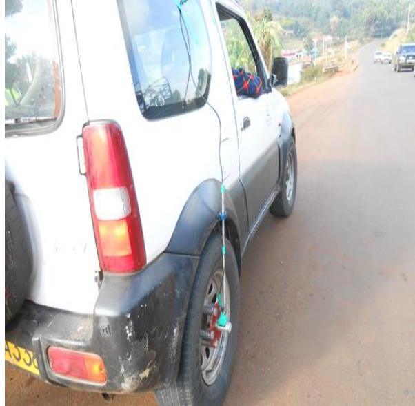
f- Wheel mounted roughness measurement
