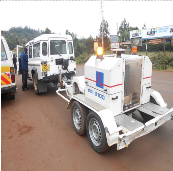
g- Standard trailer mounted FWD being operated & monitored from the Range Rover
