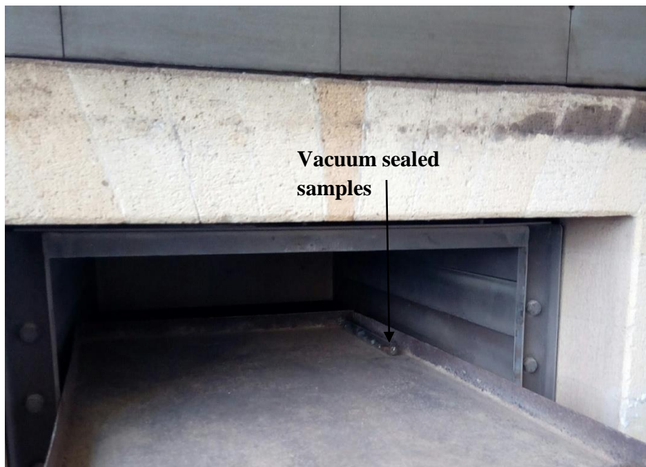
Figure 3.5: Set of vacuum-sealed samples in the Elsklo LN 2 furnace.
