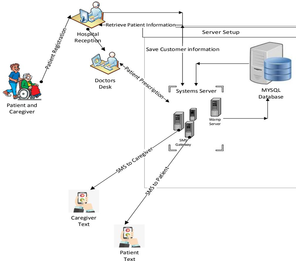
Figure 5.0: Prototype Architecture
