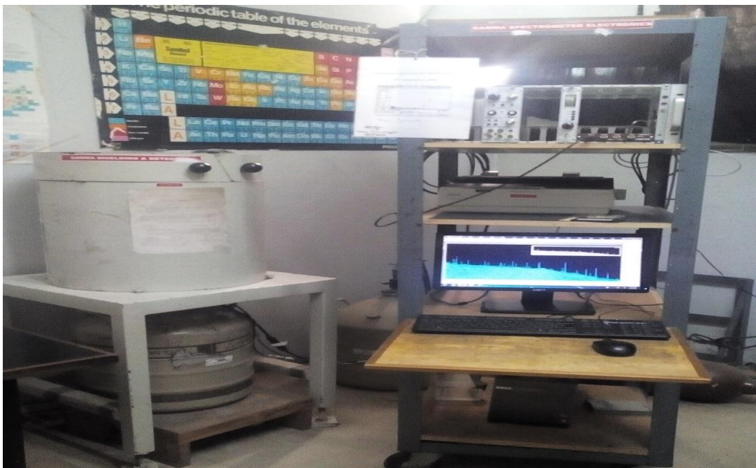
Figure 3.2: The HpGe gamma spectrometer at the Institute of Nuclear Science & technology (INST)
