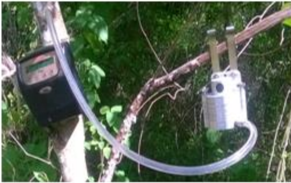
Cascade Sampler Mounted on a tree at the Apex of Kiruku Hill
