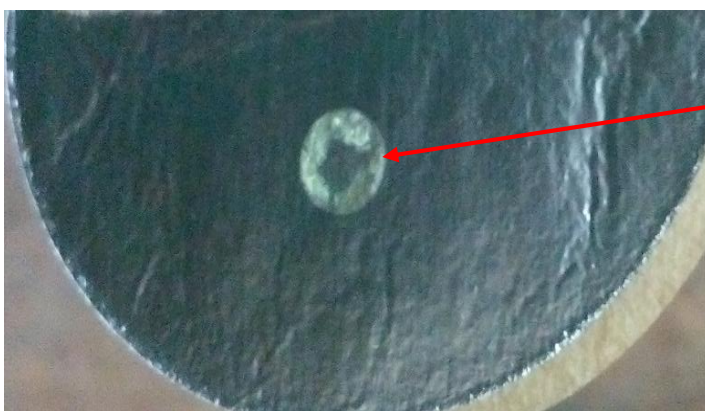
Figure 5.1: Coffee Ring on an aluminium substrate for 100 ppm of uranium using 2 \mu\text{l} aliquot with the diameter of the ring \approx 430 \mu\text{m} while thickness \approx 14 \mu\text{m} .
