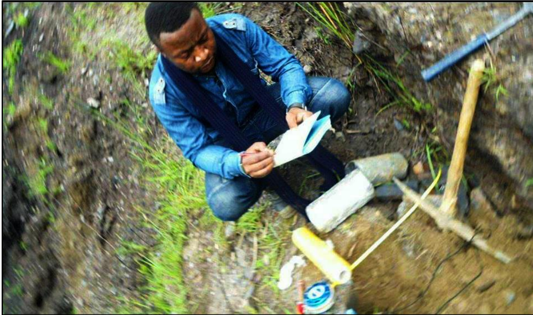
Figure 3.3 : Collecting soil samples using core cutter method.
