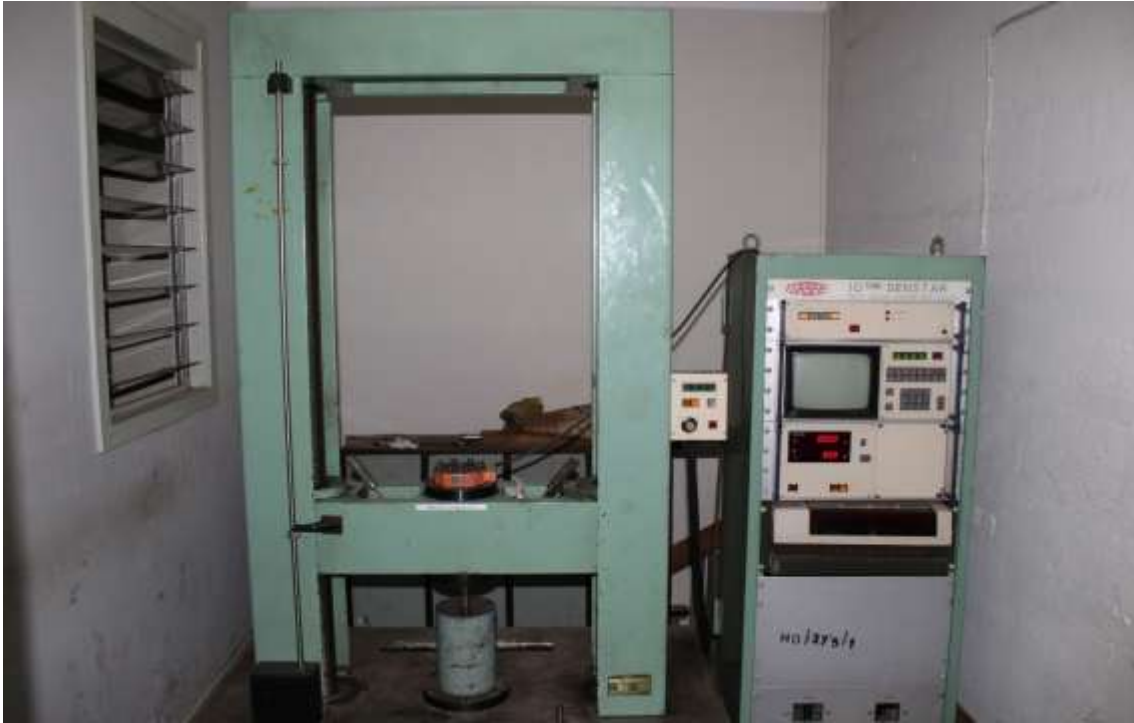
Figure 3.1: Experimental Set Up for Compressive Strength Test (Photo: Institute of Computing and Informatics, University of Nairobi).
