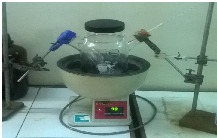
Figure 3.3: Set up used to obtain the relative humidity in thermal papers
