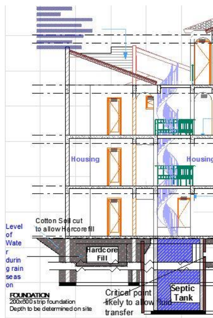
Figure 4.16B: Sketch on Critical Indications of House Foundations and Septic Tanks in the Study Area
