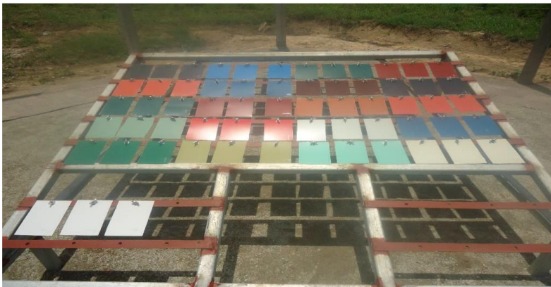
Figure 3.5: The outdoor exposure rack at Mariakani site showing pre-painted roofing sheets (Onyatta et al. , 2016).
