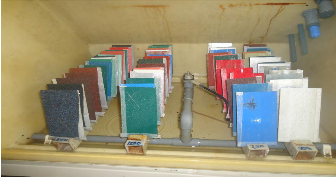
Figure 3.4: Arrangements of samples during salt spray (Fog) process (Onyatta et al. , 2016)
