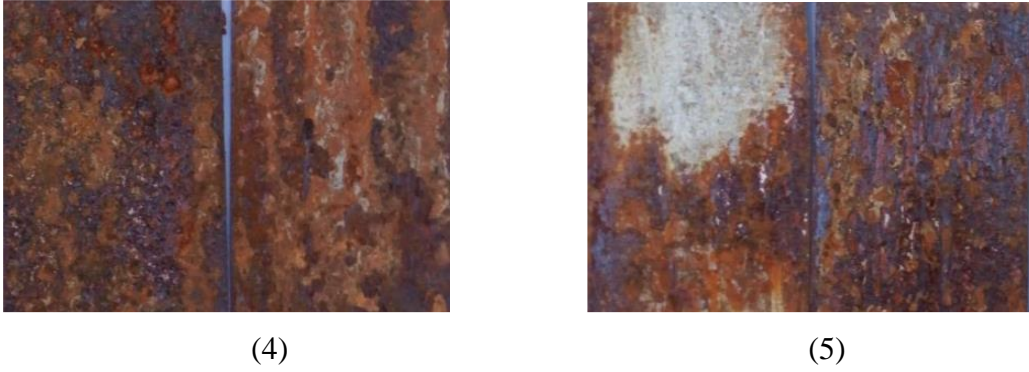
Figure 4.2: Intensity of rusting of GI samples from manufactures 4 and 5 respectively, after 28 days (672 hours) exposure in 0.073% sodium chloride and 0.289% ammonium sulphate solution.
