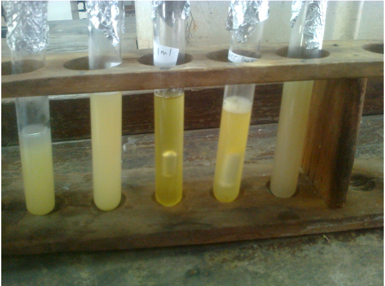
Appendix B4: photograph of samples in MacConkey's broth for coliform and E.coli assessment.
