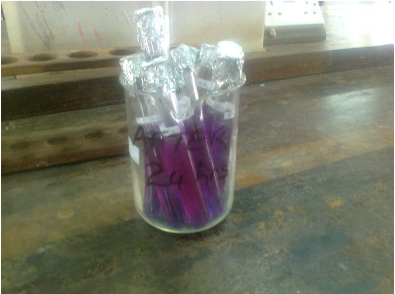
Appendix B5: photograph of samples in Mackonkey's broth after incubating for 24 hours
