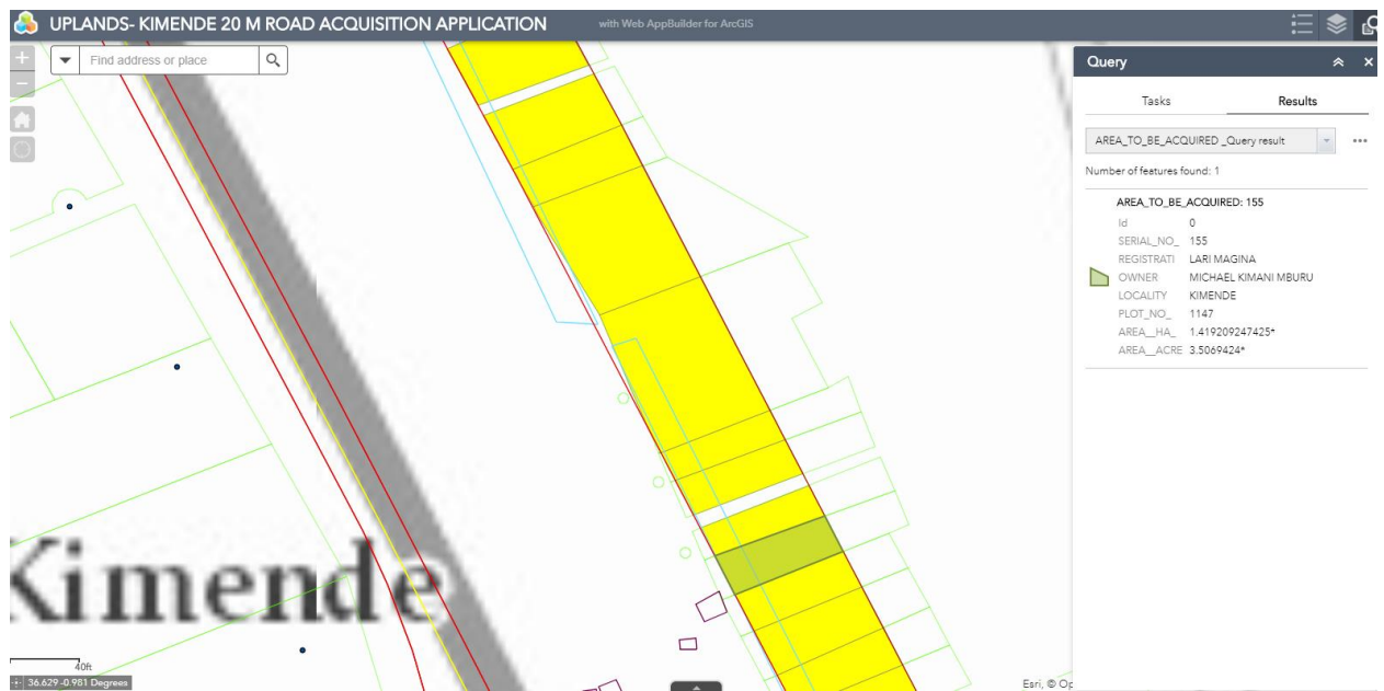
Figure 15: The Query widget enables one to obtain information from the source data.
