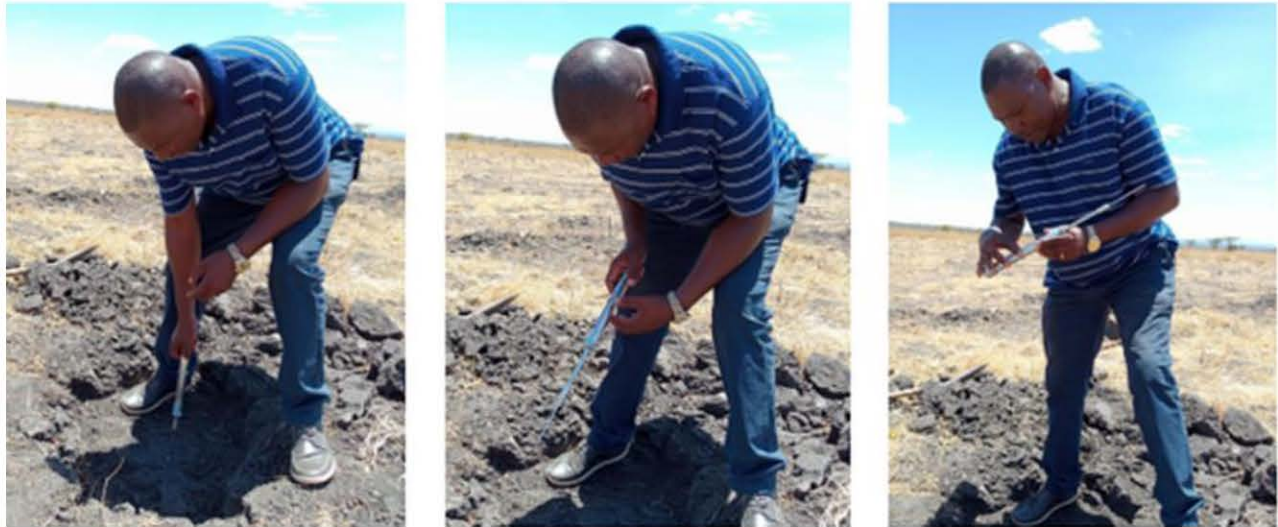
Plate 4-6 Penetration resistance measurement
