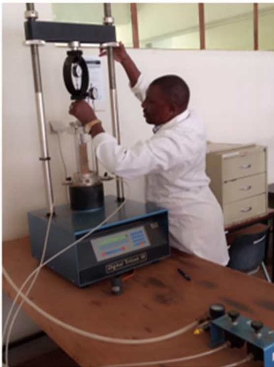
Plate 4-5 Soil sample on the triaxial machine
