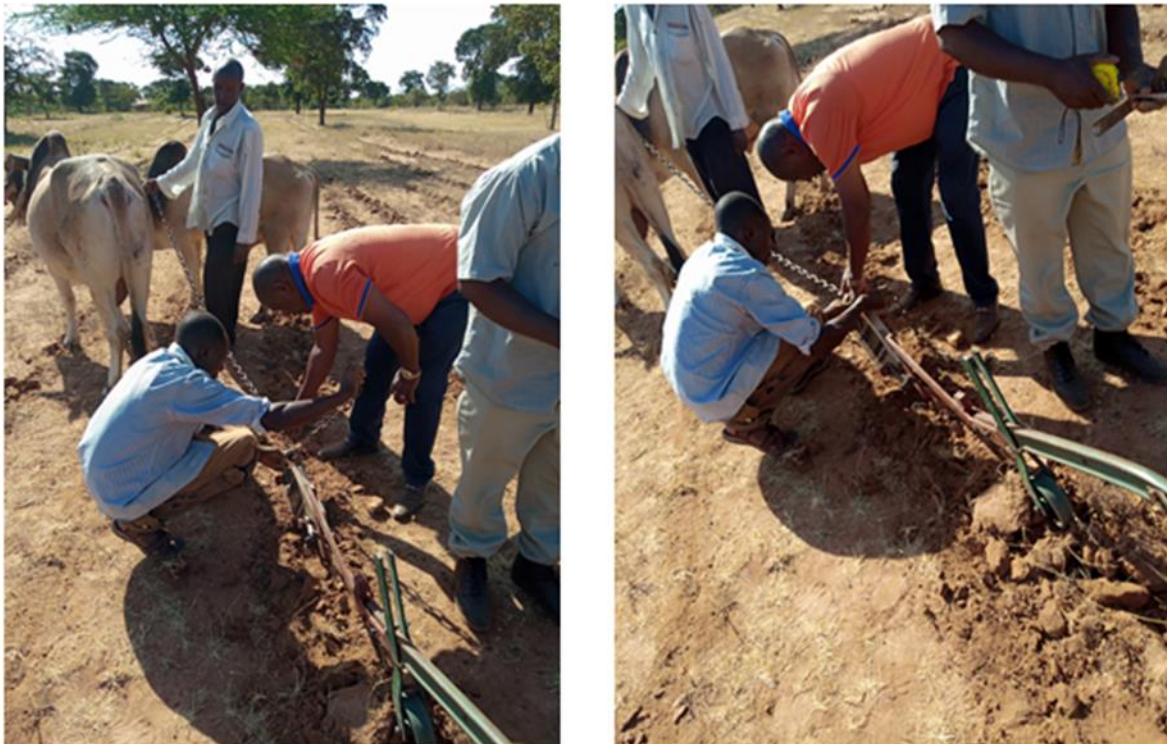
Plate 4-1 Equipment arrangement for draft data collection
