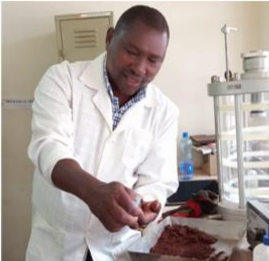
Plate 4-4 Soil sample remolding for triaxial testing
