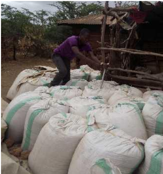
Figure 12: How to use a Sampling Probe
