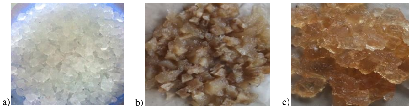
Figure 4.11. Photographs of (a) swollen cellulose-g-PAM-co-AA before burying in moist soil, (b) swollen cellulose-g-PAM-co-AA after 14 weeks in moist soil, (c) swollen PHG without cellulose after 14 weeks in moist soil
