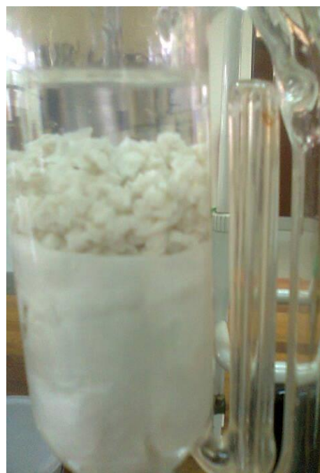
Appendix 6. a) Swollen WH cellulose-g-poly(acrylamide-co-AA), b) Soxhlet extraction of homopolymer using acetone
