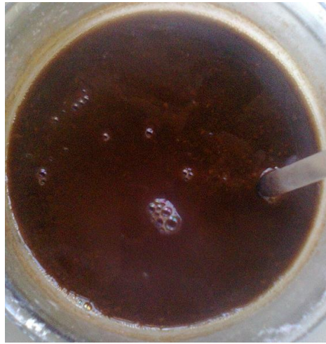
Appendix 2. a) 1 st bleaching of WH with NaOCl, b) Alkaline treatment with NaOH
