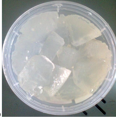
Appendix 7. a) Nano-HA powder, b) Swollen WH cellulose-g-poly(acrylamide-co-AA)/nano-HA composite
