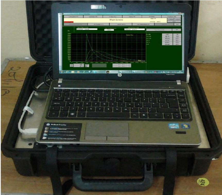
Figure 3.5 Altaix Data Acquisition System
