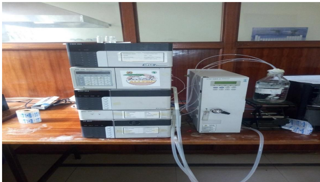
Figure 3.5: The HPLC equipment at Beekeeping Institute for analysis of sugars and HMF
