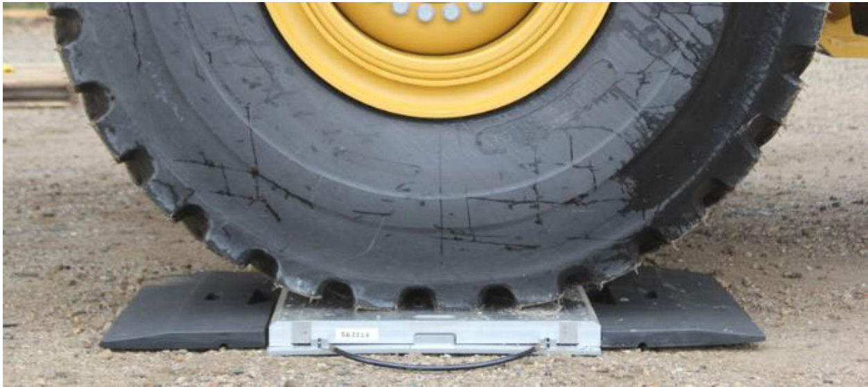
Figure 5: A single axle-weigher
