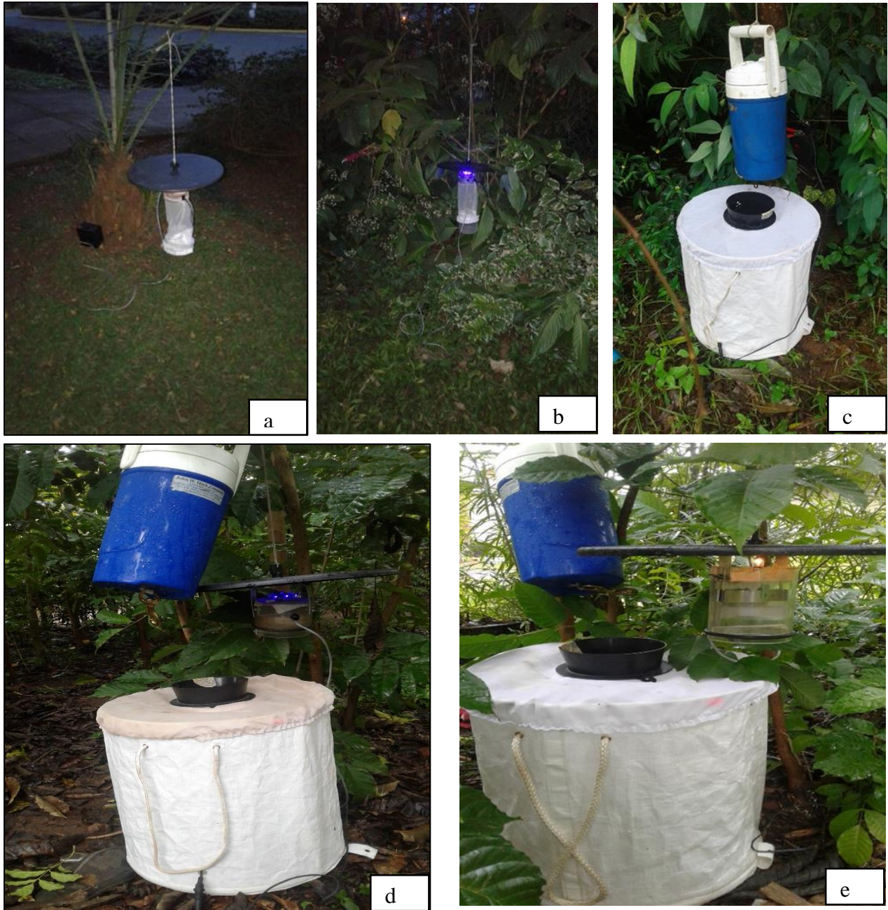
Figure 5: Traps panel including modifications used in experimental evaluation of Ae. aegypti catches: a) incandescent CDC model light trap, b) Ultra violet CDC model light trap, c) BG-S 1 trap, d) BG-S 1 trap + UV light, e) BG-S 1 trap + CDC incandescent light
