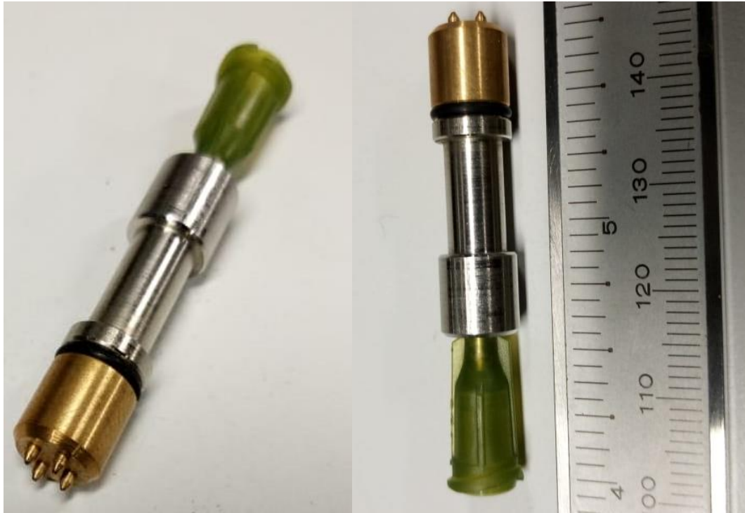
Figure 4.47: Photos showing a single nozzle with four orifices.
