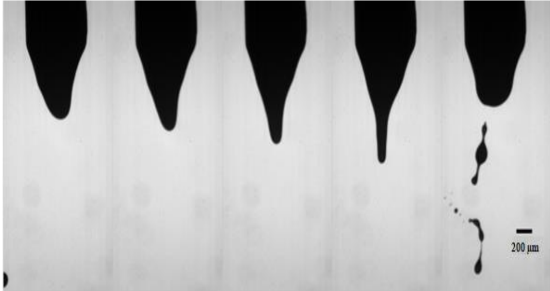
Figure 4.6: Electro spray sequence for IMF solution with 30% w/w solid content at a flow rate of 5 \text{ mL h}^{-1} and an electric potential of 13 kV. The frequency of the mode is \sim 2.3 \text{ ms} .
