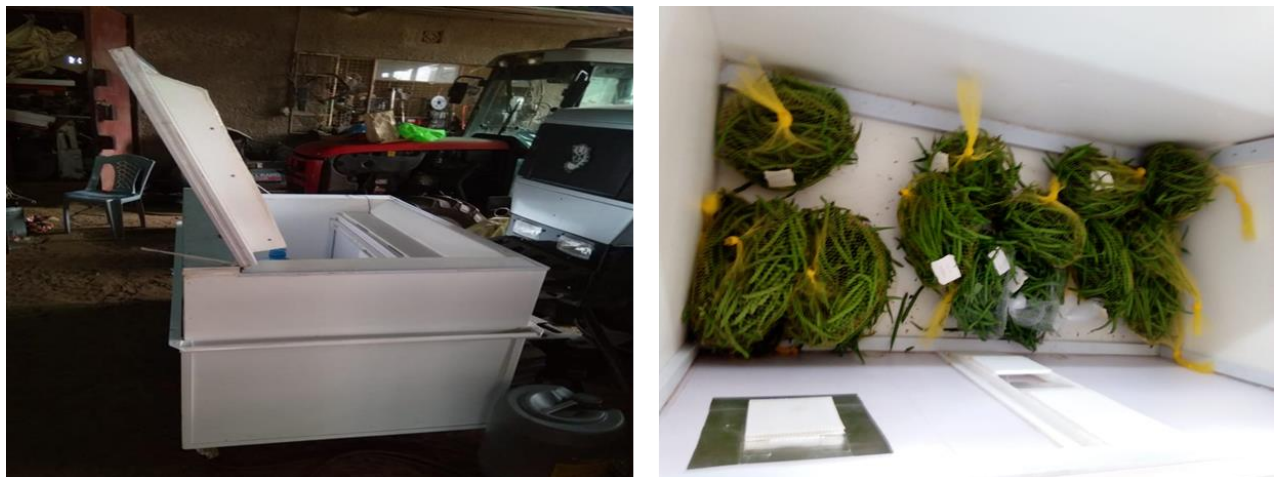
Figure 6. 4: L-The upper portion of the solar cooler and (R)- packed French beans stored in the cooler
