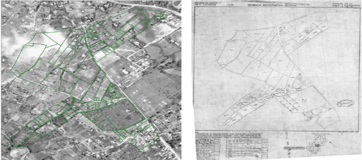
Figure 2. 3 Left marking of un-rectified aerial photographs; Right product – PID after tracing from marked photographs (Siriba et al., 2011)
