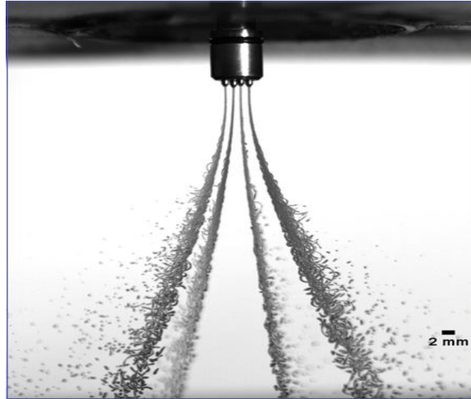
Figure 4.55: An image stack showing droplets dispersion obtained at a flow rate of 2.1 L h -1 and an applied potential of 19 kV (solid content = 55% w/w)
