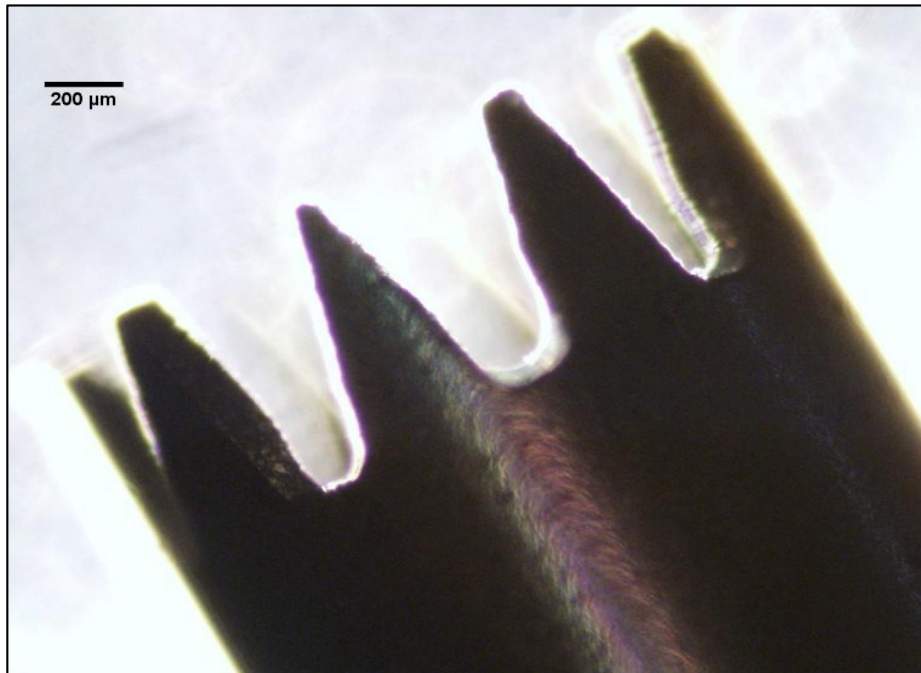
Figure 4.44: A photo of the serrated nozzle
