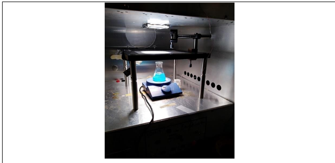
Figure 3.1. Photocatalytic degradation of Methylene blue setup
