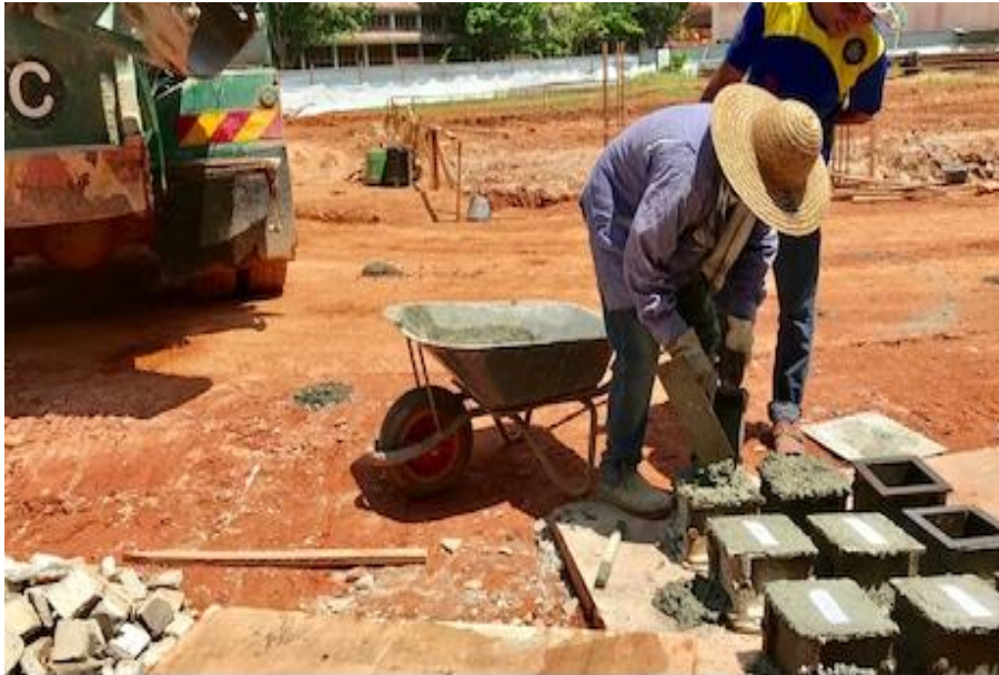
Plate 2.4: Placing fresh samples in cube moulds.
