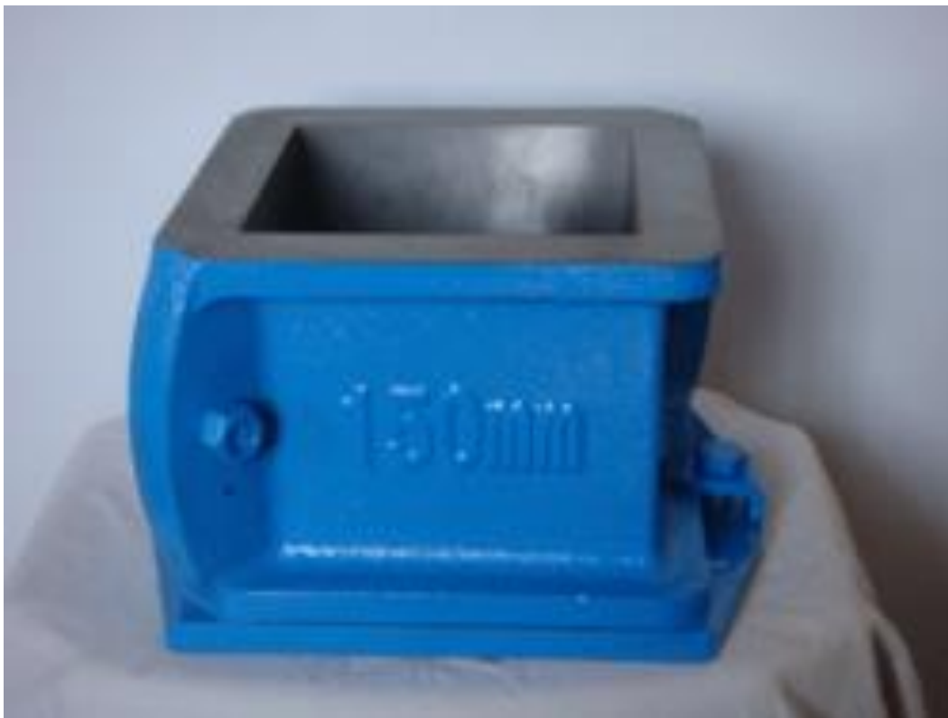
Plate 2.3: A standard Mould (150mm x 150mm x150mm)
