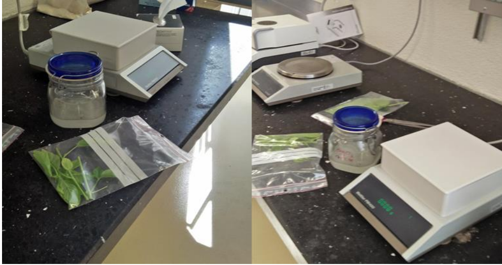
Plate 4-5. Harvested leaves and humidity jar used for the sorption experiment
