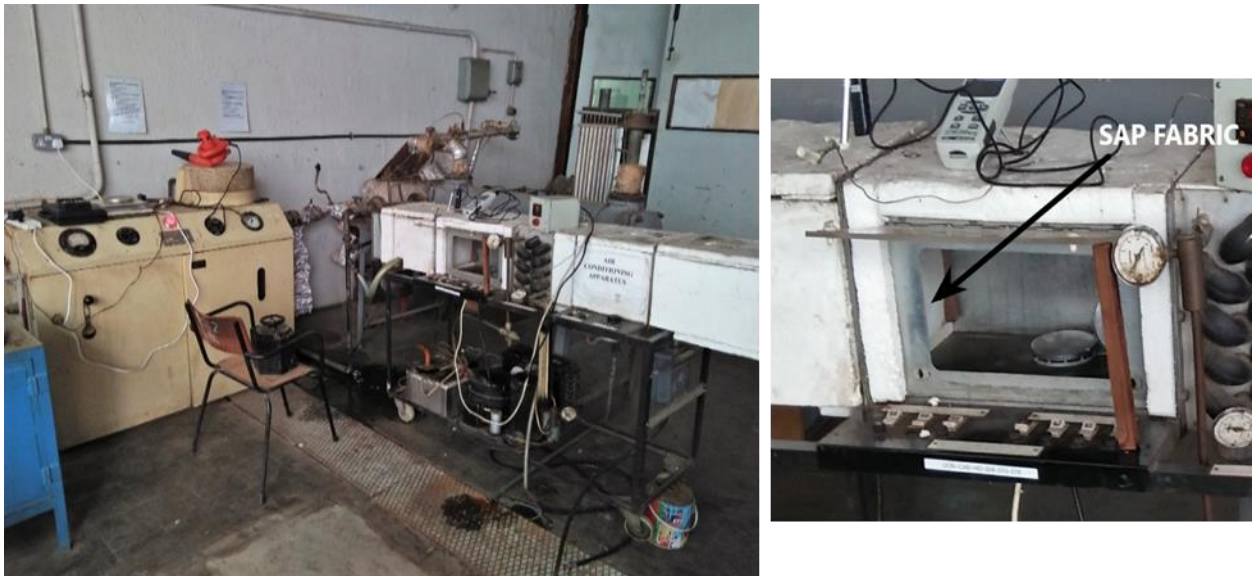
Plate 4-2. Experimental set up photo for super adsorbent polymer characteristics.
