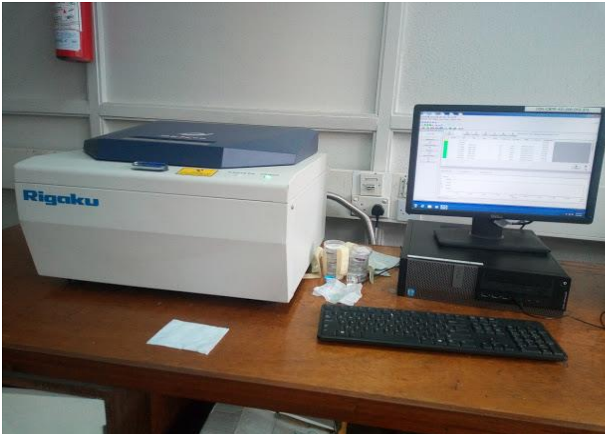
Figure 3.4: Rigaku NEX CG EDXRF spectrometer at the Physics Department
