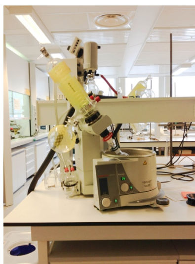
Figure 3-7: Rotary evaporator set up used for drying extracted lipids at near vacuum conditions
