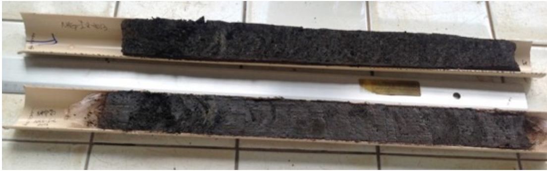
Figure 3-2: Sediment cores from Lake Nkunga comprising two short sediment cores NKG-I-1-2013 and NKG-I-2-2013 each approximately 45 cm. One half of the sample was subsampled every 1 cm for sample preparation and analysis while XRF scanning was carried out on the other half of the core.
