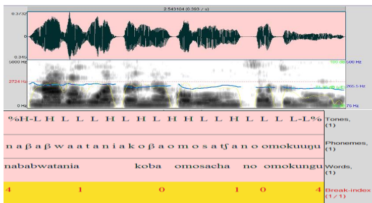
Figure 6: Audio waveform, F0 contour and ToBI label windows for /naβaβwatania koβa omosafʃa no omokunʃu/ produced by a 9-year-old female
