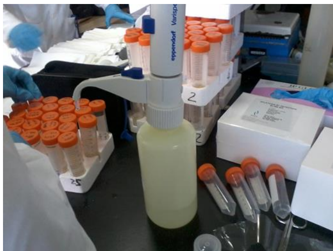
Figure 4-2 Aflatoxin extraction using 80% acetonitrile
