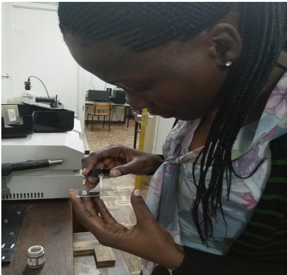
Figure 4. 3: Spreading of the conductive silver paste on the microscope glass slide
