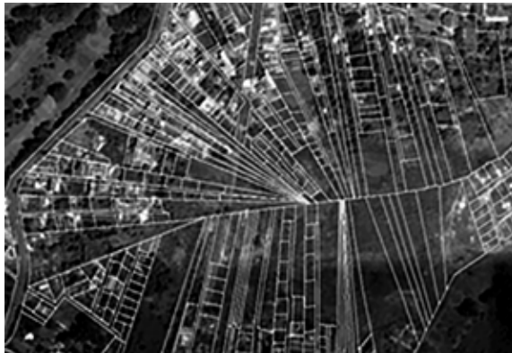
FIGURE 8 Narrow parcel configurations in Kiambu Town Source: Cadastre digitized from Survey of Kenya RIMs 2017
