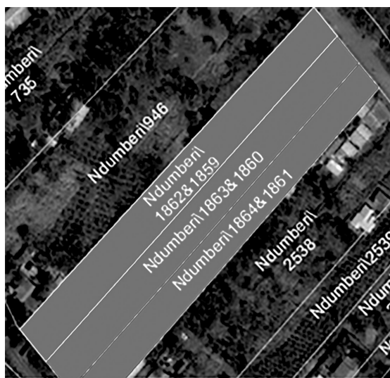
FIGURE 10 Illustration showing parcels having more than one number Source: Cadastre digitized from Survey of Kenya RIMs 2017
