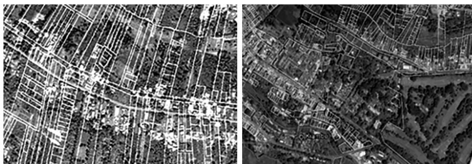
FIGURE 4 Sample of inconsistencies found when cadastre layer was overlaid on an Ortho-rectified image Source: Cadastre digitized from Survey of Kenya RIMs 2017
