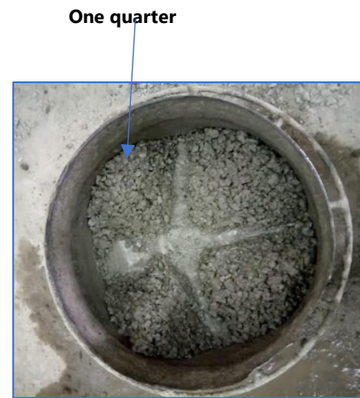
Figure 3.8: A quartered batch of fresh concrete.
