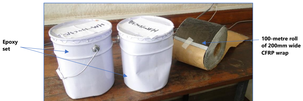
Figure 3.13: Carbon fibre wrap and epoxy adhesive.
