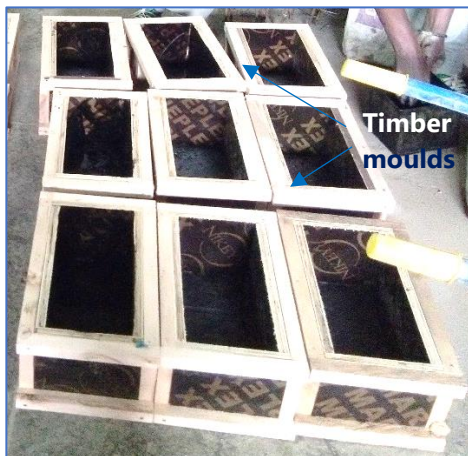
Figure 3.5: Setup for the manufacture of plain concrete specimen.
