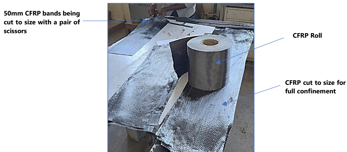
Figure 3.14: A pair of scissors was used to cut the CFRP to the required sizes.
