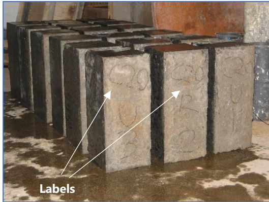
Figure 3.9: Samples after removal from the water bath.
