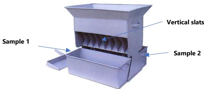
Figure 3.7: A riffle sample divider.
