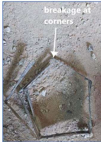
Figure 4.38: Failure was characterised by rupture at the corners.
