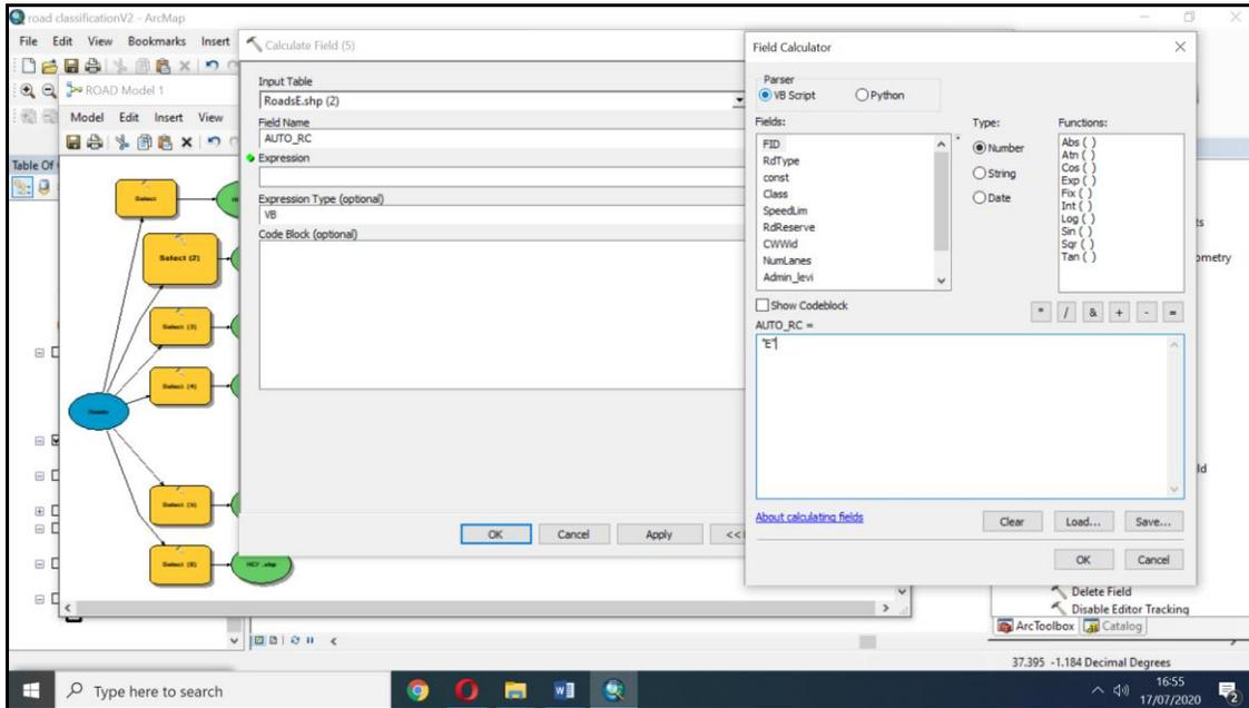
**Figure 3.12: Adding a field in the classified roads layer inside model**
