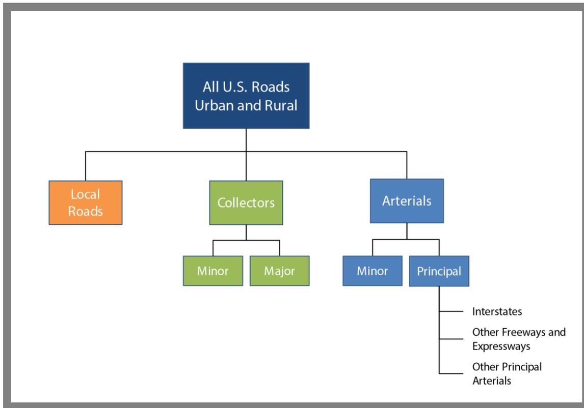
**Figure 2.1: US Highway Functional Classification System Model**
